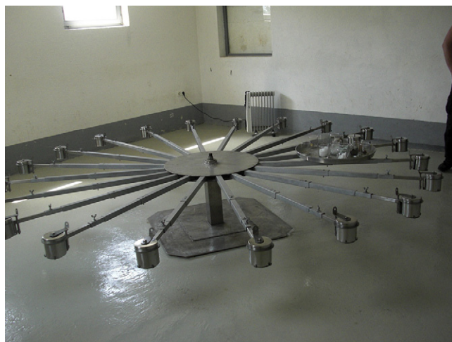
Figure 3 Carousel with 24 arms used in the advanced training of mine detection dogs at GTC.
