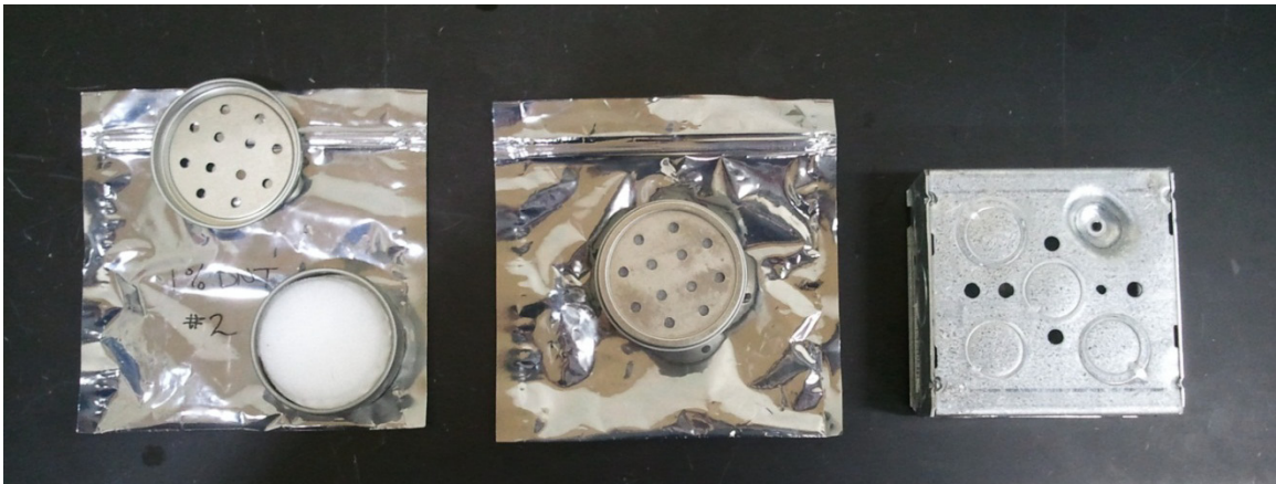
Figure 55. NIST training aids. From left to right: open training aid where particles are placed, closed training aid, standard metal box in which the NIST training aids were hidden for canine trials
